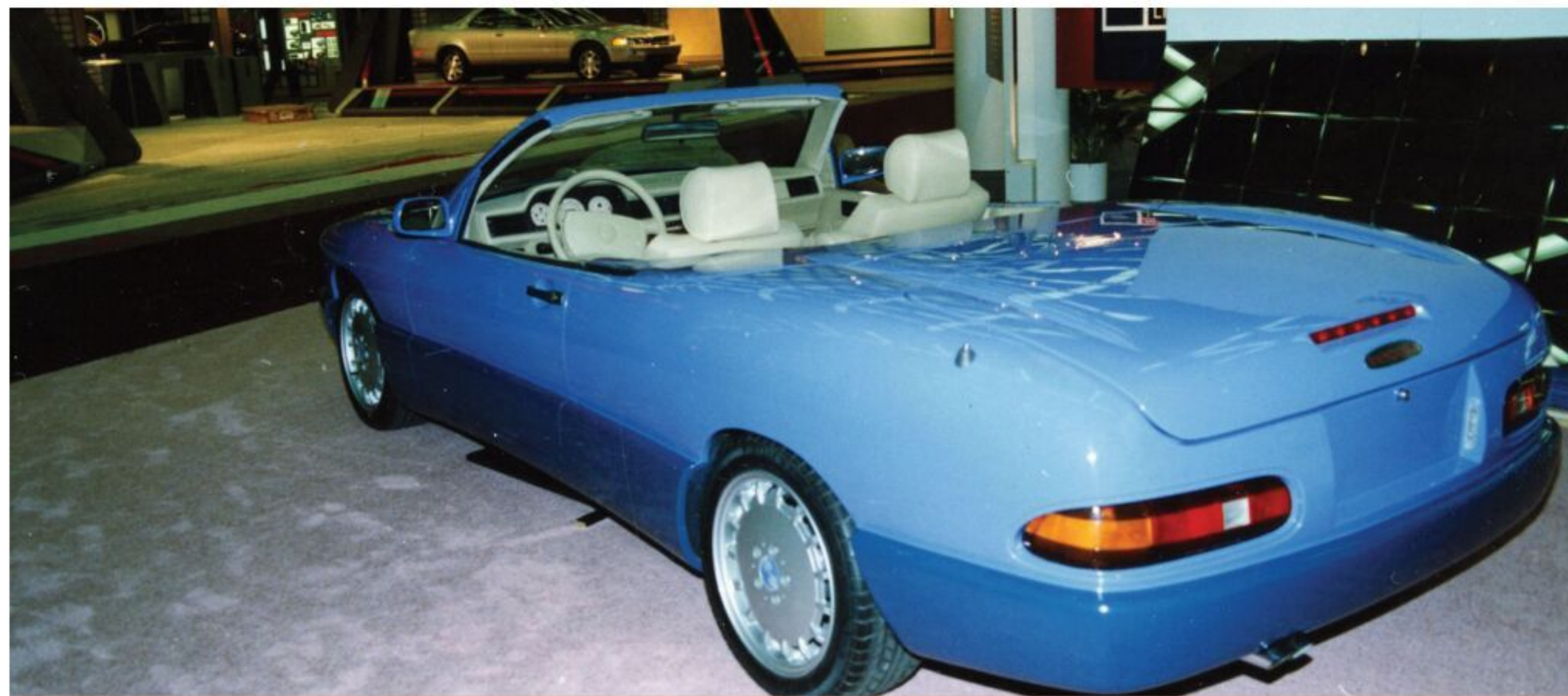
Pandora's new body parts were made from carbon graphite and kevlar reinforced plastics.
