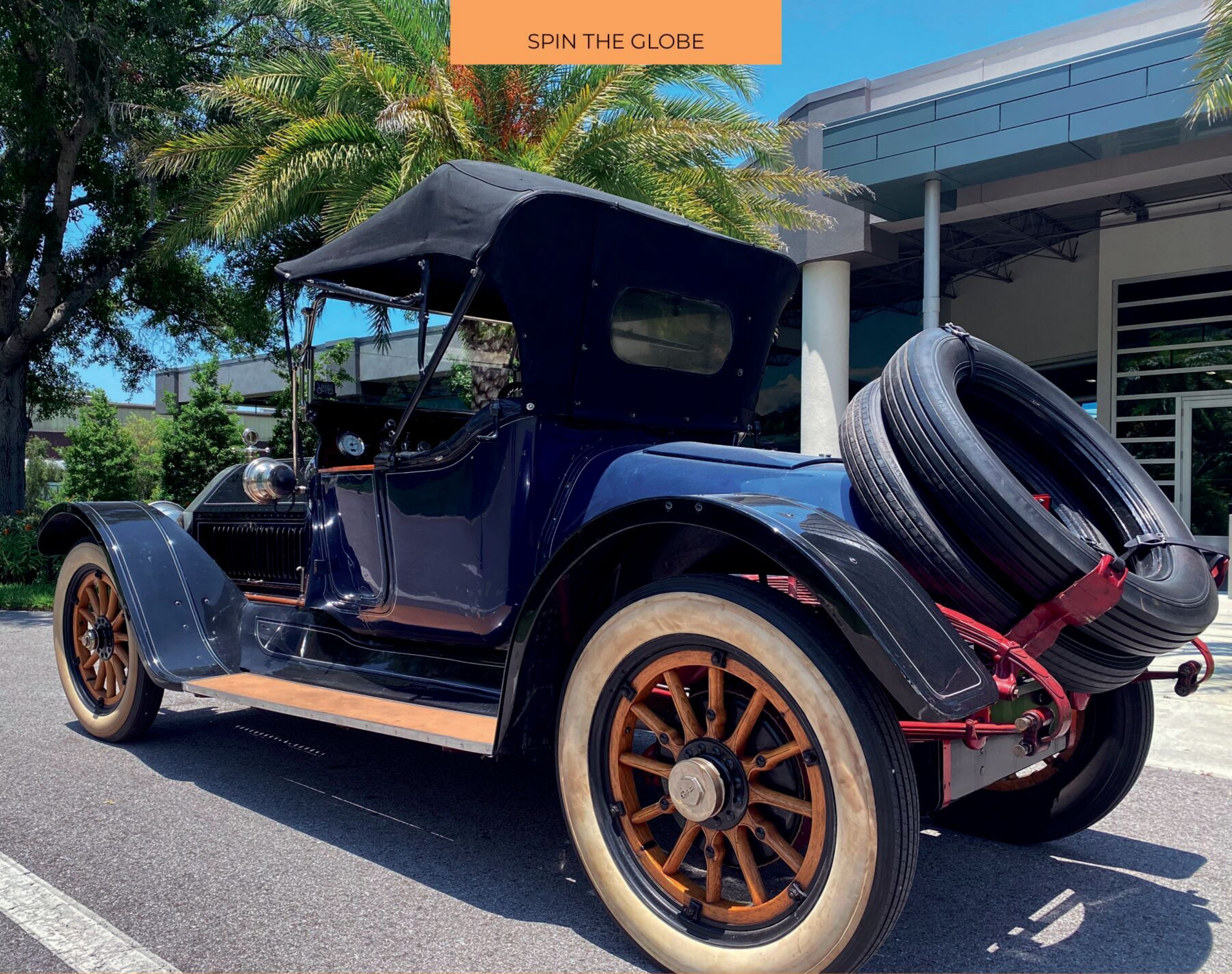
The two-seater roadster body was built on a 132-inch-long (3.35 meters) long wheelbase.
