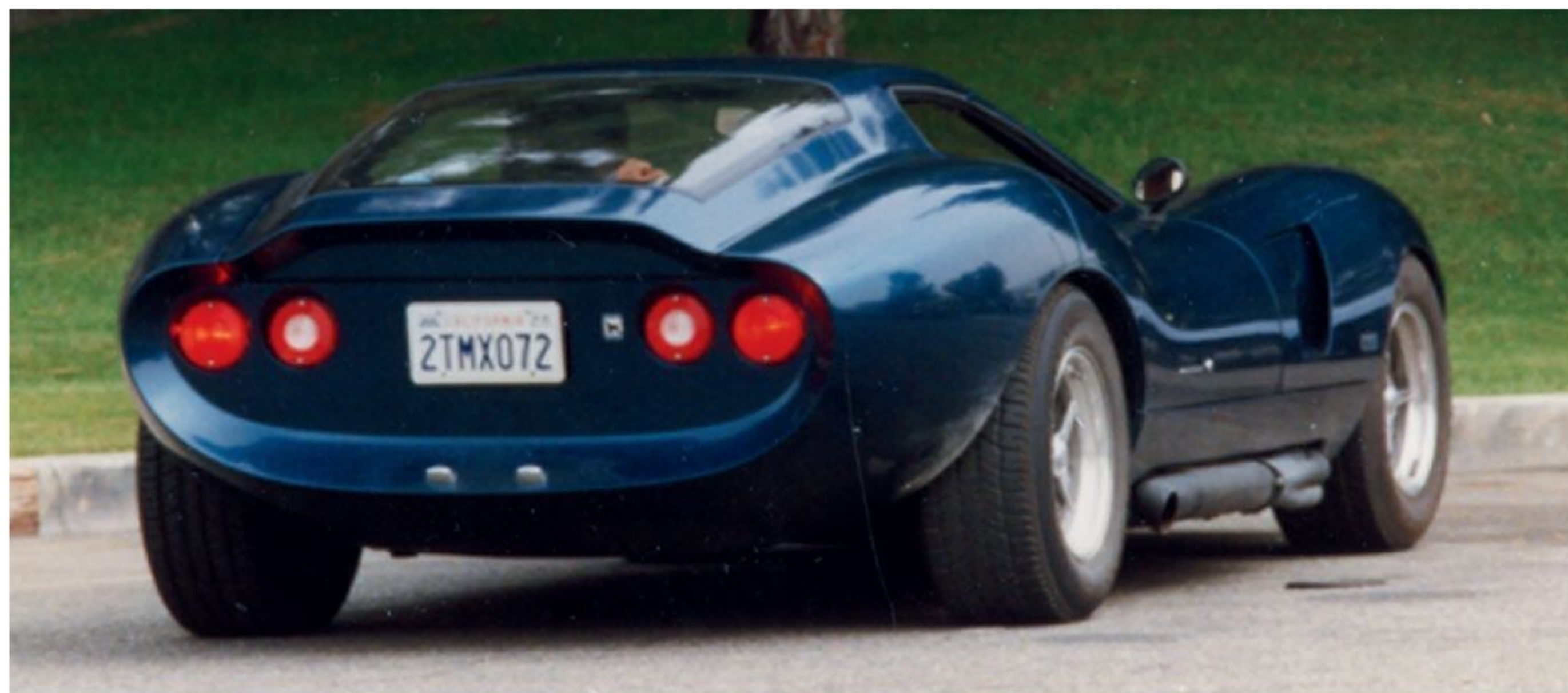
A stock Chevy V-8 powered the fiberglass-bodied Afghan.
