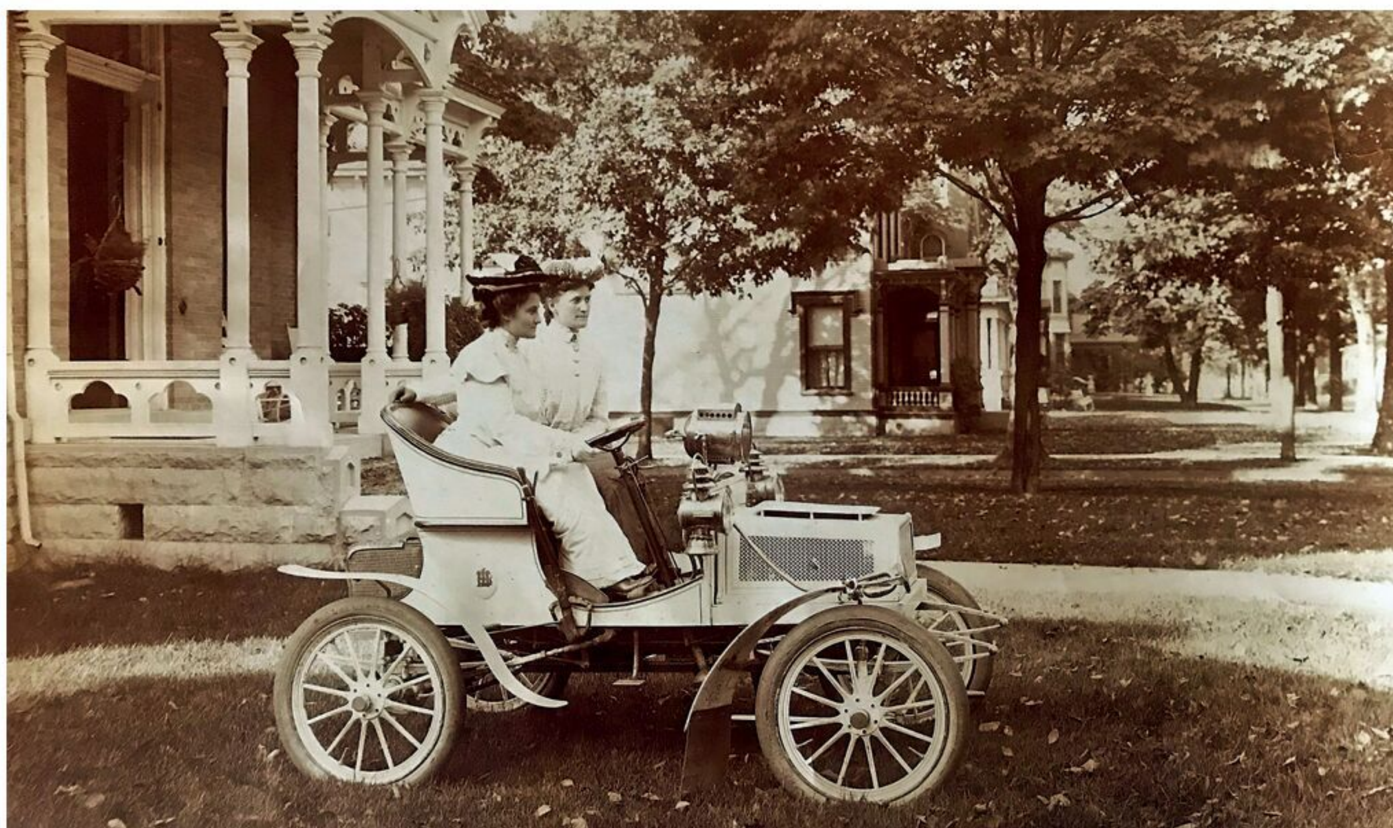
A 2-cylinder air-cooled Mitchell runabout from 1904. Pictured are Mary and Helen Lewis, daughters of the company's founder, William T. Lewis (Lewis Miller).
