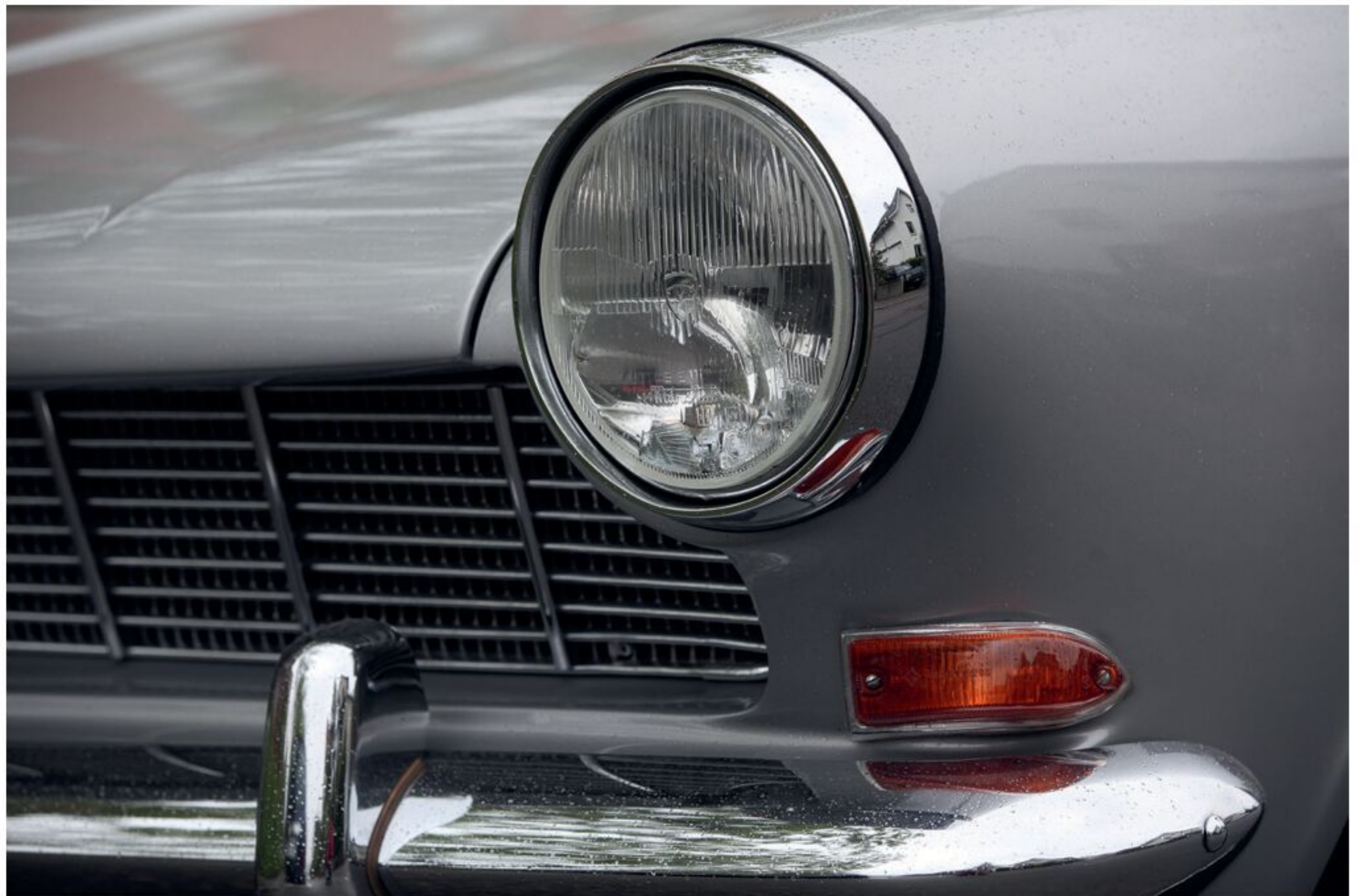
Bumpers, bumperettes (mounted upside down), and turn indicators taken from the Kadett.
