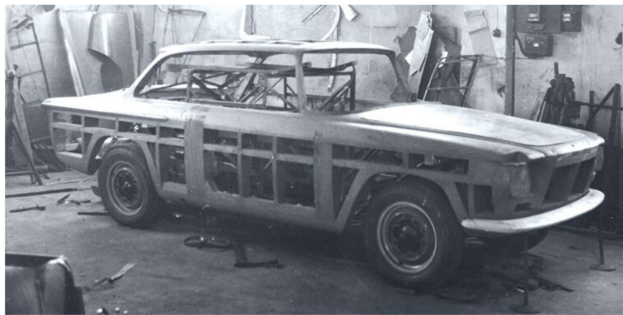
The wooden buck for the Volkswagen Italsuisse Sedan "Sun Valley" in the Studio Tecnico Pietro Frua in Torino (Photo: Pietro Frua, Frua-Family-Archive Roberto Rigoli).
