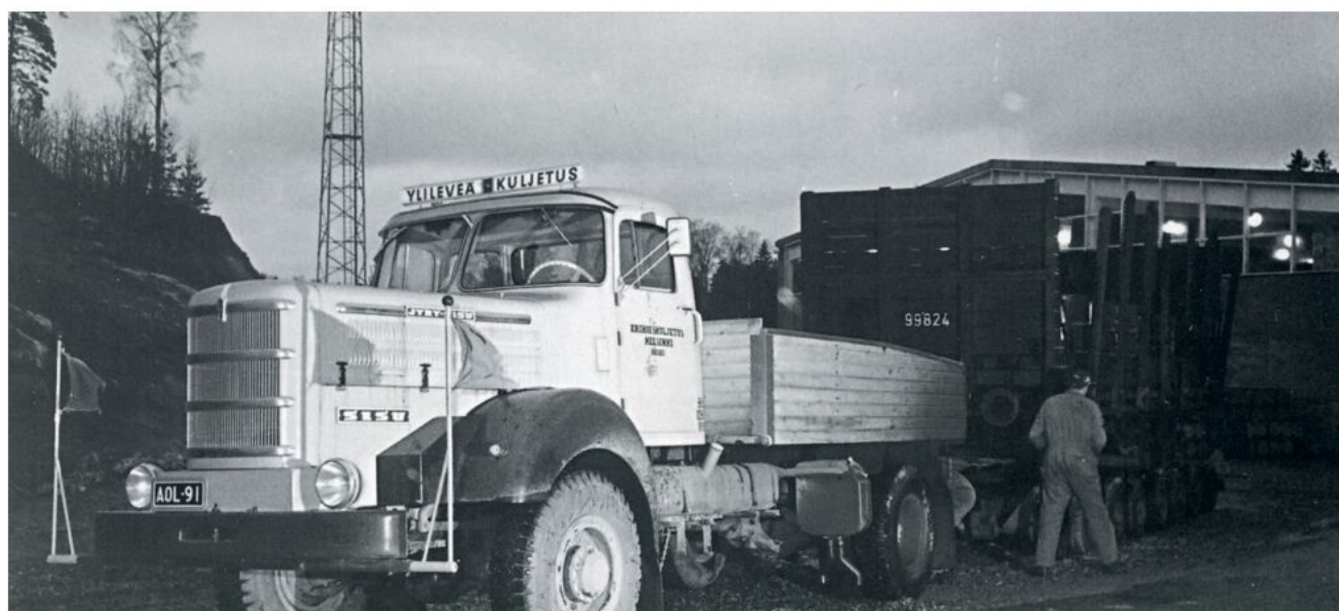
A heavy-duty K-405ST 4x4 nicknamed the Jyry-Sisu from 1959. Jyry means rumble or other loud, low sound from the distance.
