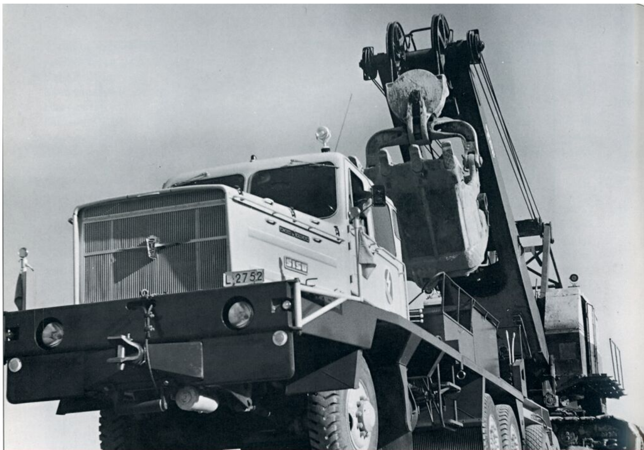
The 1961 Sisu K-50SS is probably still the largest street-legal road vehicle manufactured in Scandinavia. It was powered by a 300-hp Rolls-Royce F6-TFL engine and had a towing capacity of 38 tons.
