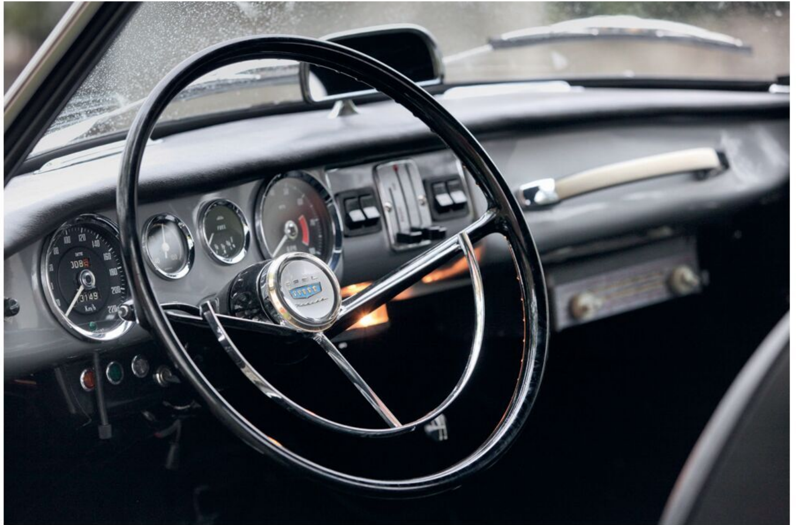
Round instruments taken from the Lotus Elan, which Frua rebodied as a coupe for the 1964 Geneva Show.
