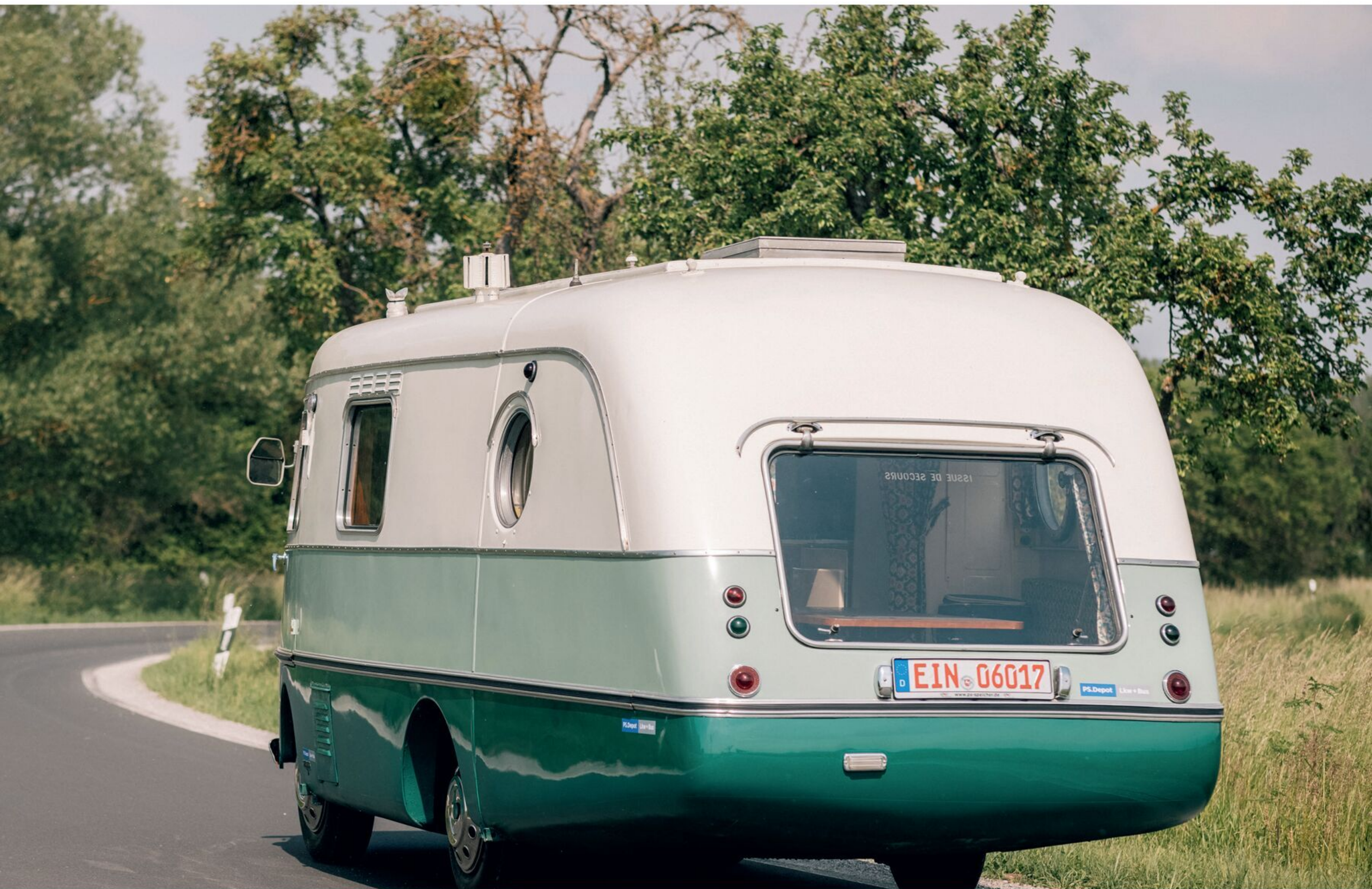
There is a two-meter extension at the back which houses the camper compartment.
