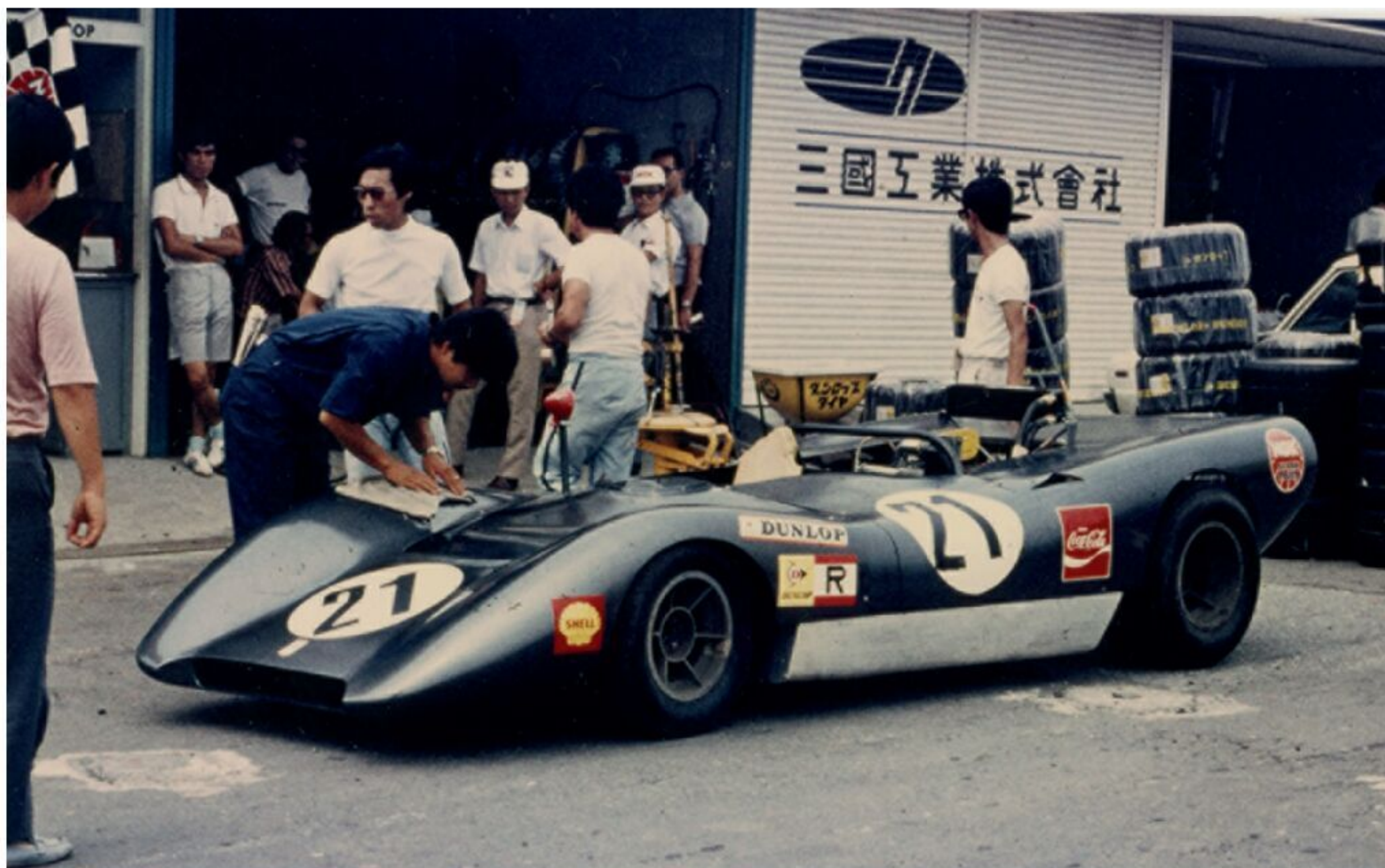
The Day & Night Mk V, the first version of Watanabe's Lycaon used a Brabham chassis.
