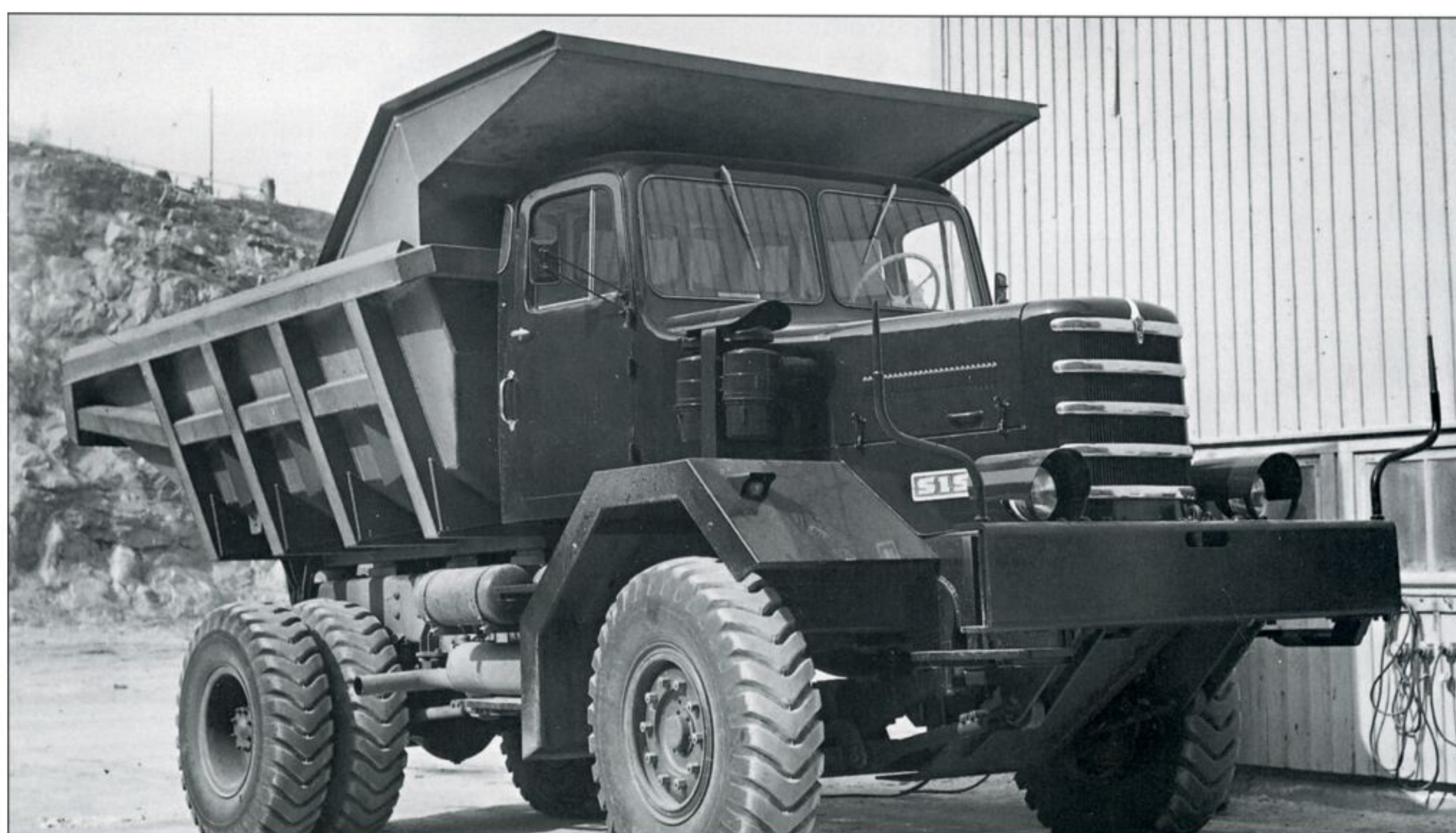
The Sisu K-36SS dumper was in production between 1958-1960, powered by a Rolls-Royce diesel engine.
